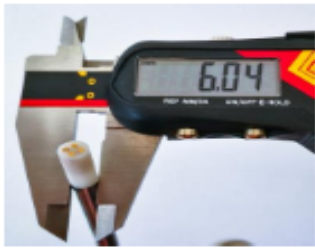
Figure 1. Tip of the 5.5 mm probe used. (Photograph by JCMG).
