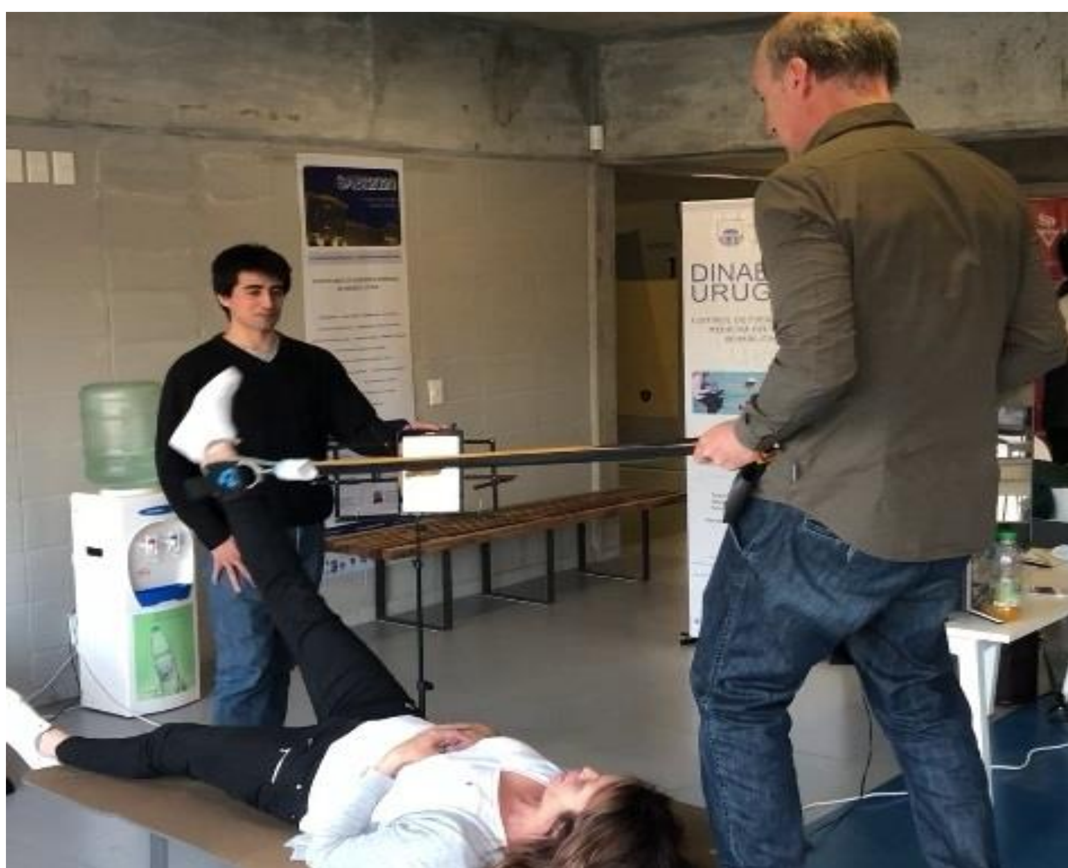
Figure 1. DINABANG® instrument during isometric force evaluation. Supine position of amateur sportsperson with hip at 60° and the leg is pushed towards 0°, tending to extend the hip with fully extended knee.
