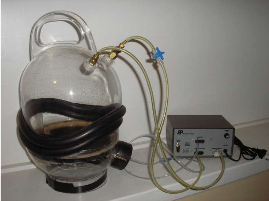
Fig. 3. ABDOPRE 2007 bell applied to the phantom and rear part of the cabinet [9].
