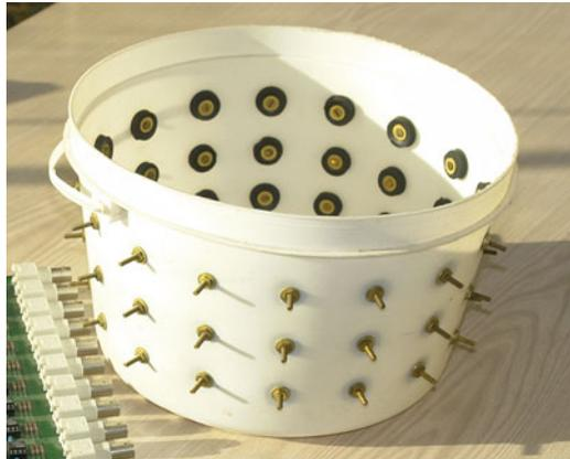
source (Saulnier 2004) controlled by one of the codec output signals, proportional to a DSP-originated 16 KHz sinusoidal wave. We suggest to include the test RC “phantom” within the actual EIT instrument, to be available as “self-test” or “self-calibration”.
