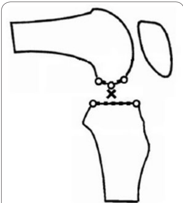
Figure 1. Schematics of knee bones with point of contact determination. Five anatomical points are defined at the extremities of the tibial plateau and along the femoral condyle. The Tibio Femoral Contact Point (TFCP) is defined as the midpoint of the shortest segment between femur and tibial plateau. Modified from the original figure by Bernardes [27].
