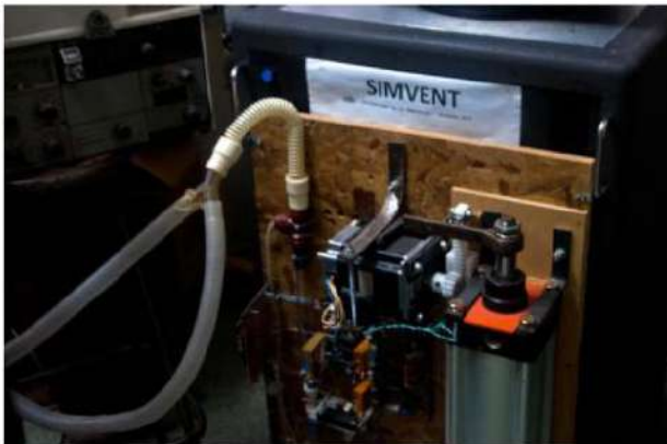
Fig. 2 - Implementation of a second SIMVENT prototype. Note the "Y" tube which is used to connect to Mechanical Ventilators (MV)
