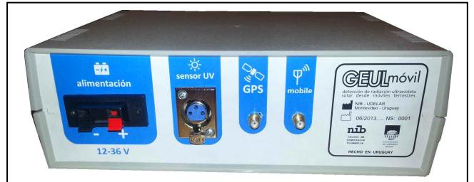
Fig. 3. GEULMóvil quick-fit connector panel.
