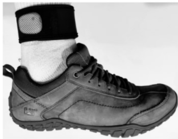
Figure 4.1: PARKIBIP elastic ankle band with the IMU sensor. Image from [1]
