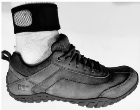
Fig. 1. PARKIBIP elastic ankle band with the IMU sensor. Image from [22].
