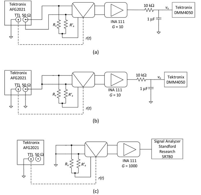
Fig. 6. Experimental setups used for characterizing the FD synchronous demodulator in order to estimate (a)  $G_{DD}$ , linearity, and quadrature rejection, (b)  $G_{DC}$ , and (c) spectral density of the noise voltage. The second block on each block diagram corresponds to the circuit under test.
