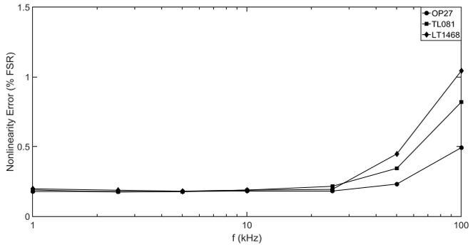
Fig. 8. Nonlinearity error expressed as a percentage of the FSR at different frequencies for the three op-amps.
