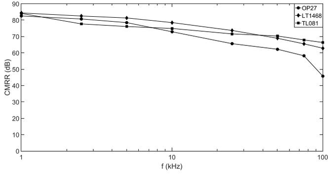
Fig. 7. CMRR of the FD synchronous demodulator measured at different frequencies for the three op-amps tested.
