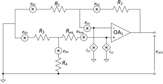
Fig. 5. Semicircuit used to estimate the PSD of noise at the output of the FD synchronous demodulator.
