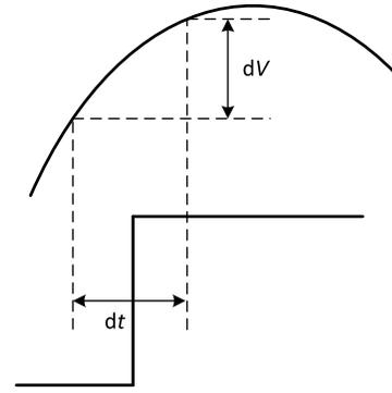
Fig. 4. Voltage error versus aperture jitter [26].
