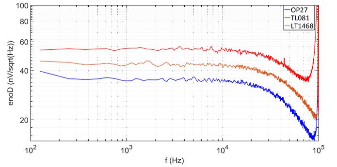
Fig. 10. Spectral density of the noise voltage of the proposed circuit when it was implemented with the three op-amps presented in Table I. Switching frequency = 100 kHz.
