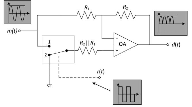
Fig. 1. SE switched-gain amplifier used as a synchronous rectifier.
