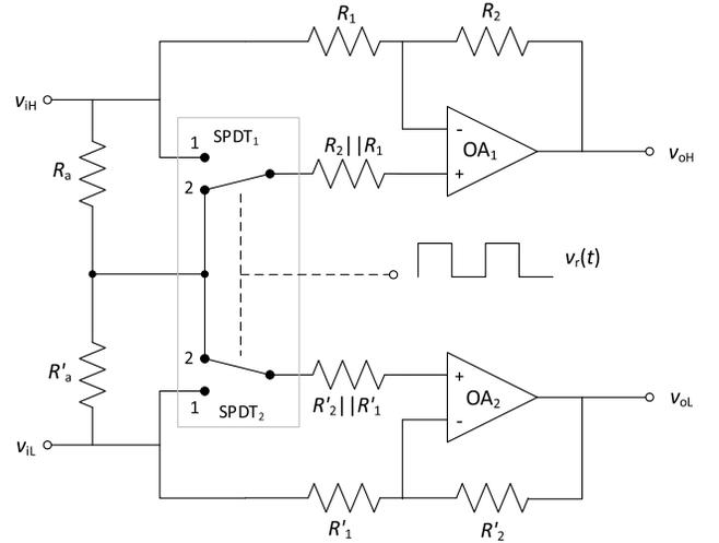
Fig. 2. Proposed FD synchronous demodulator for ac signals.
