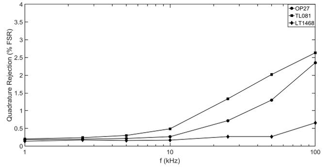
Fig. 9. Quadrature rejection expressed as a percentage of the FSR at different frequencies for the three op-amps.
