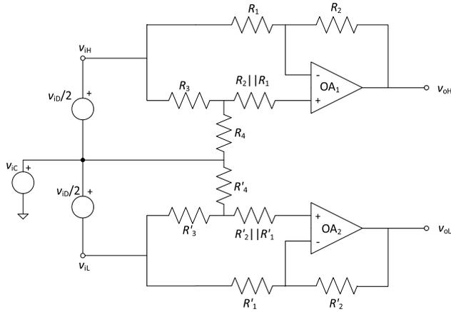
Fig. 3. Equivalent circuit of the FD synchronous demodulator used to estimate the CMRR.
