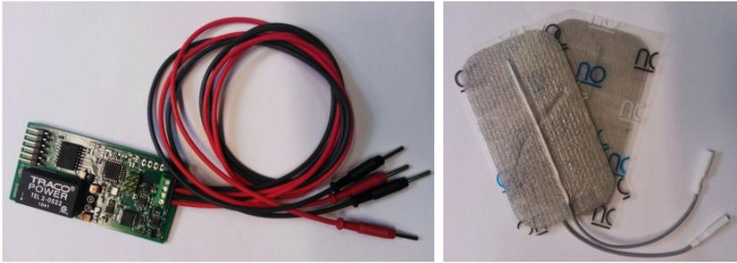
**Figure 2.9.** OpenEBI measurement electronics [V] and a pair of self-adhesive 5 x 9 cm rectangular silver/silver chloride (Ag/AgCl) electrodes.
