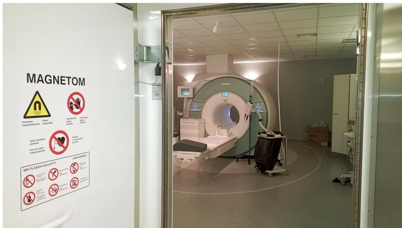
**Figure 1.3.** A 1.5-Tesla MRI scanner with a 70 cm wide bore photographed from the door of the radio frequency (RF) shielded MRI room. This particular scanner, located at Meilahti Helsinki University Hospital, was used in [III].
