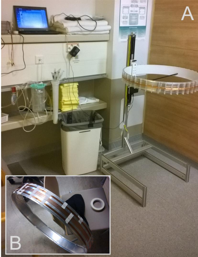
**Figure 2.4.** The second version of the BELA instrument used in [III]. The photograph (A) is taken at the Helsinki University Hospital, Meilahti. For the measurements, the coil was attached to a stand and connected to a laptop via a USB (Universal Serial Bus). Photograph (B) shows the coil winding under design. The aluminium frame also worked as an electrostatic shield as in [II]. The Figure is adapted by the author from [II].
