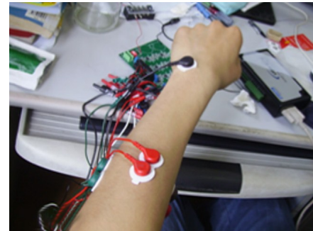
Figure 1: EMG electrodes placed on the skin surface [4]
