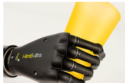
Figure 6: I-Limb ultra, from the company Touch Bionics, is capable of being programmed with a wide range of gestures. Other similar models are also available. [18]
